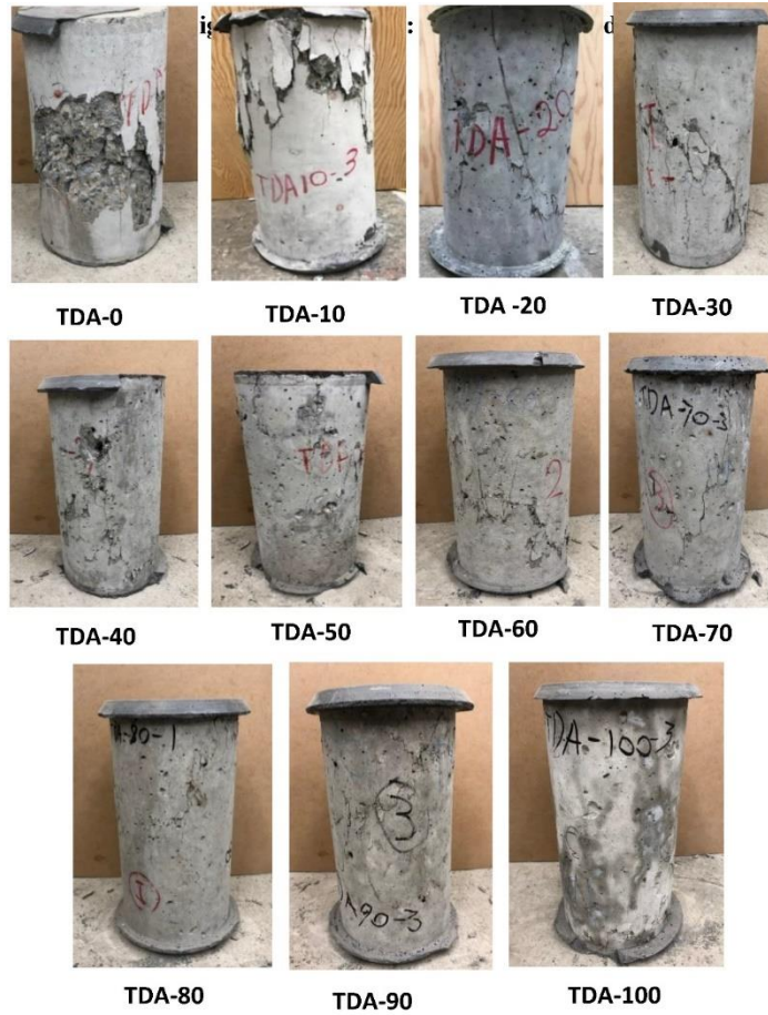
Figure 3: Cylindrical concrete specimens after failure
